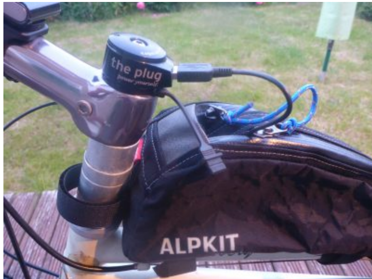
The Plug USB charging port running off the dynamo hub
